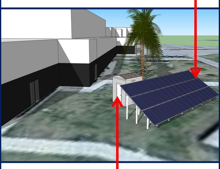
The SOLAR EQUIPMENT ENCLOSURE houses the inverters, batteries, and charge controllers.
